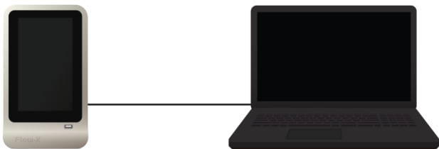
Figure 9-1 Direct Ethernet connection without switch
