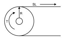
If the load above requires torque T pound-inches and is driven with a pulley on the motor shaft a with a radius of R inches, the side load imposed on the motor shaft is T/R pounds. If the motor shaft is connected to a sprocket for a chain drive, R is one half the pitch diameter of the sprocket. If an external load with a weight of W pounds is also being supported by the motor shaft above, the total side load on the shaft is:
