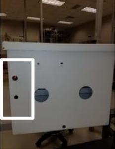
A photograph of a white metal enclosure. A white rectangular box highlights two antenna holes on the bottom left side of the front panel.            |
