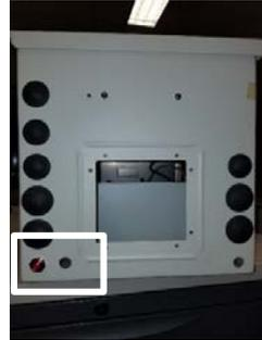
12. Remove the black protective plug from the antenna hole in the enclosure.
