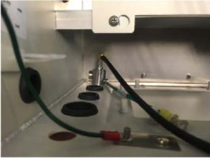
15. Attach the ground cable to the ground post (see number 2 in the picture below).
