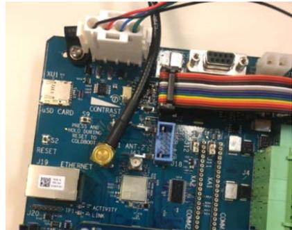
3. Attach the plug-to-jack adapter to the straight SMA fitting of the cable.
