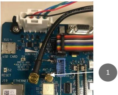
The Wi-Fi antenna installation is complete.
