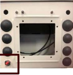
A photograph of the back of a white metal enclosure. A red rectangular box highlights a red and black antenna hole located at the bottom left corner. |
