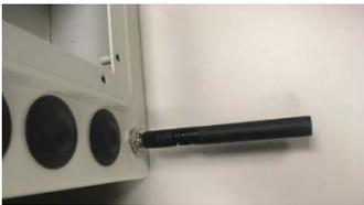
20. Attach the terminator plug to the board ANT-2, connector (J43). (see number 1, below).
