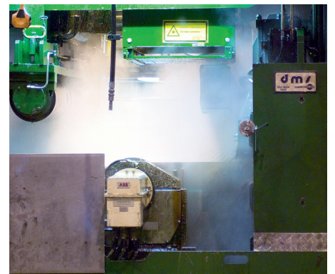
Stressometer Flatness Control System combined with Millmate Strip Tensiometer in a temper mill.
