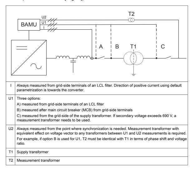
Recommended nominal primary measurement range of the current transformer for BAMU I measurement is 130% of the nominal AC current ( $I_N$ ) of the IGBT supply unit. Secondary current is 1 A.
