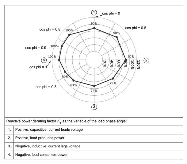
The amount of reactive power affects also the loadability of the converter. The basic rating is given for negative active power and the output current needs to be derated if there is reactive power or if the active power is positive. The figure above shows the derating factor depending on the phase angle of the load current.
