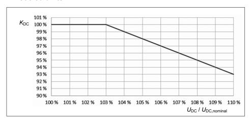
DC link voltage derating is 1% for each 1% of DC link voltage boost above 103%. Derating factor can be calculated with following equation:
