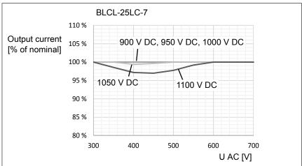
Select the derating curve according to the LCL filter type that is used with the desired IGBT supply unit type. Voltage derating factor depends on grid voltage and DC link voltage. To be able to calculate the derating factor, the DC link voltage requirement must be known. For calculating the DC link voltage, see section DC link voltage requirement (page 26).
