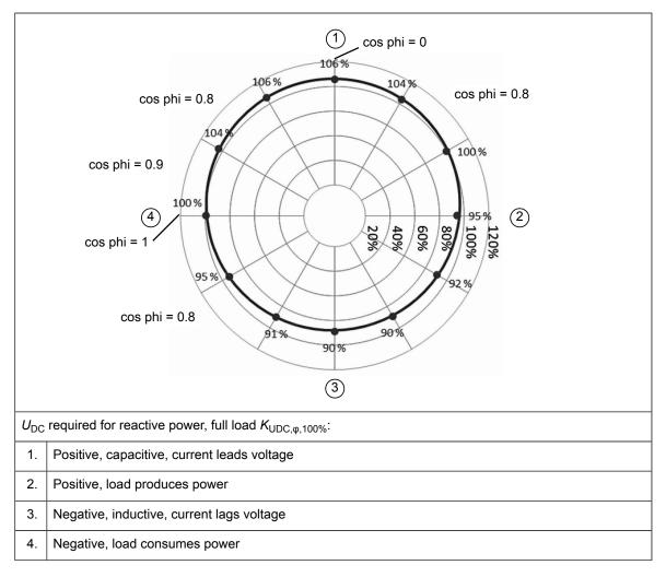
A linear fit equation can also be used for the loading between no load and full load.
