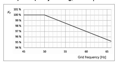
Above 50 Hz the output current is derated 0.3% / Hz.
