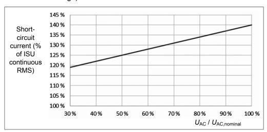
The curve is based on the nominal (continuous) current rating of the IGBT supply unit. Current available from the grid converter is less especially with lower grid voltage. See section *Voltage derating, factor*  $K_U$  (page 20).
