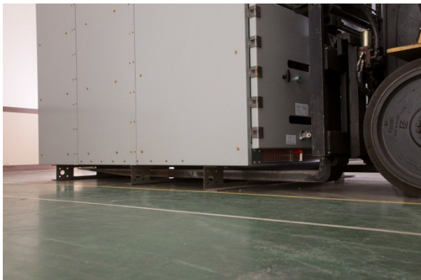
Complete fork penetration of all 3 shipping channels
