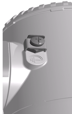
Figure 1 External protective earth (PE) terminal
