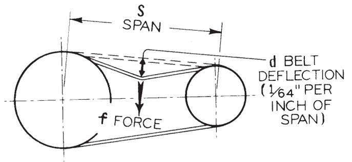
1. At the center of the span apply a force (perpendicular to the span) large enough to deflect the 1/64, for every inch of span length. For example, one deflection of a 100 inch span would be 100/64 or 1-9/16 inches.
