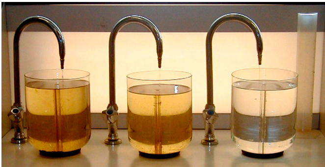
Figure 2 Change in river-water color through the coagulation process
