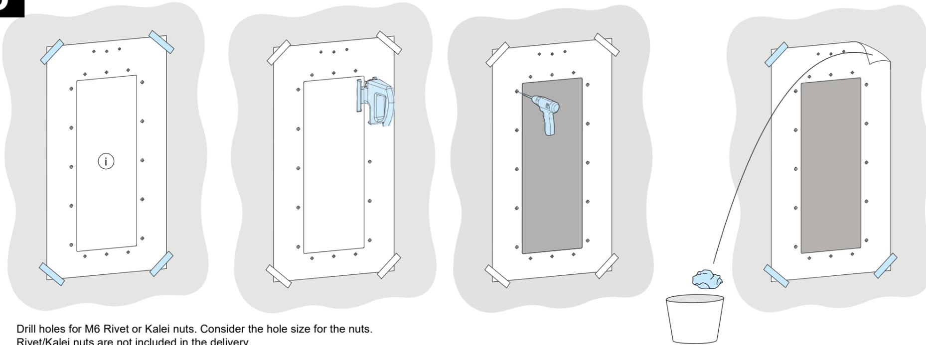
Drill holes for M6 Rivet or Kalei nuts. Consider the hole size for the nuts. Rivet/Kalei nuts are not included in the delivery.
