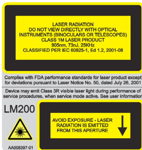
Figure 2- 1. LM200, Class 1M Laser Safety Label
